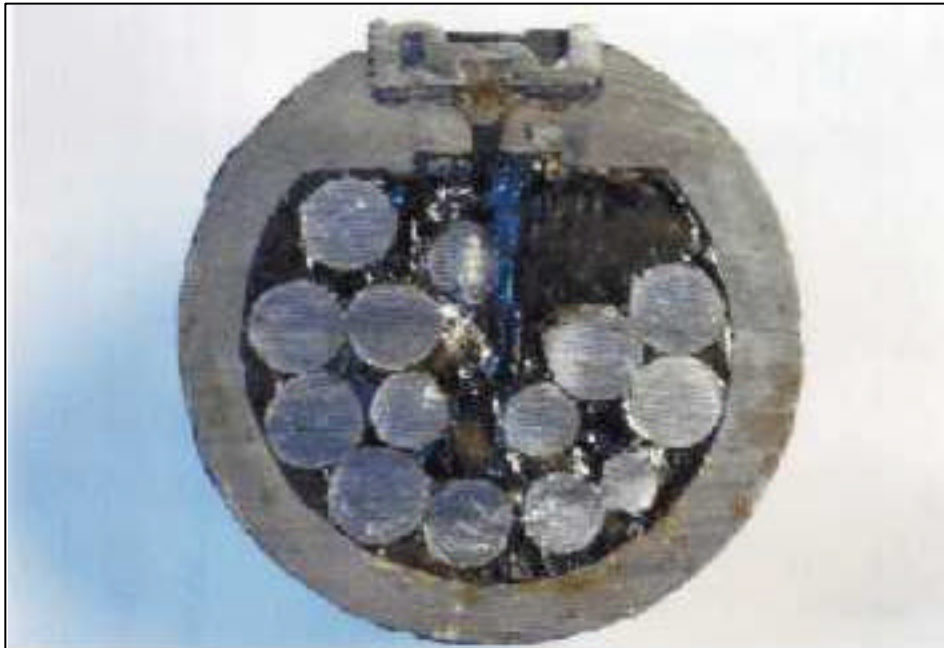
Illustration 49: A cross-section of the 12-pounder spherical case showing the fuse, powder chamber, and .69-caliber round balls in a matrix. Douglas Scott
